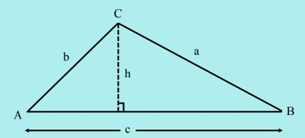
We can always create right triangles by drawing an <u>altitude</u> from any vertex.
