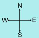
(b) A <u>bearing</u> is always measured from north, in a clockwise direction. The values are from 000 to 360 (but less than 360).
